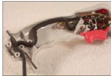
Photo 9: Routing the PTT cable.
