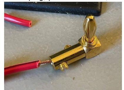
Figure 3: Before coating solder joint with sealant
