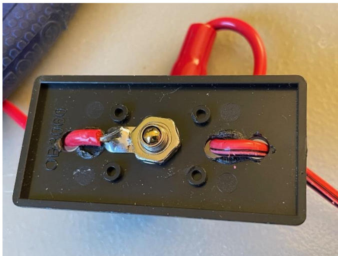
Figure 2: Before coating solder joint with sealant
