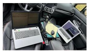
My GreenCube station requires two laptops – a MacBook to run my satellite tracking software (SatTrack) for controlling the radio and the antenna rotator, and a Windows laptop to run the unique GreenCube SoundModem and Terminal programs.
