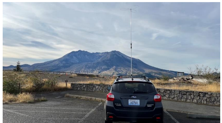
Operating Location 1 near Johnston Ridge Observatory at Mount St. Helens NVM in Skamania County. The antenna was installed only while parked but meets height restrictions for legal motion. Band changes required swapping loading coils. This is the 20-m configuration with a home-built loading coil.
