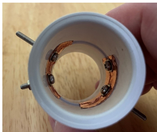
Figure 3, The PVC coupling used for the driven element. Coax from the radio connects to the short studs
